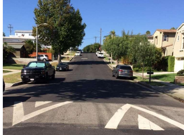
Image for Note 7: This speed hump is located on a section of the block where the grade is less than 8% but as far up the hill as possible
