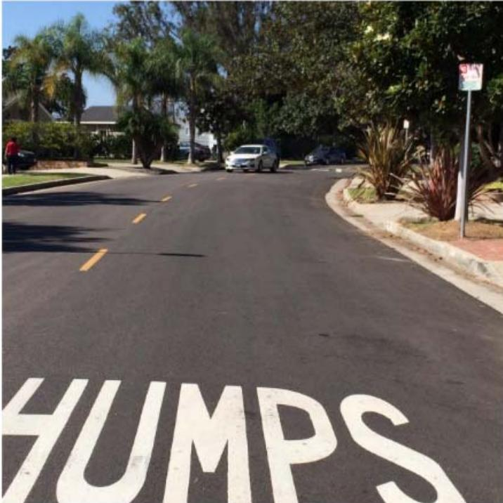
**Note: The speed hump at the top of this image is visible from the “HUMPS” marking at approximately 200 feet away**
